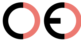
False CE Mark (too far)
